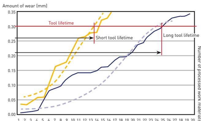
A graph created of tool life based on the acquired data and analysis results. Contributed to the reduction of tool replacement.
