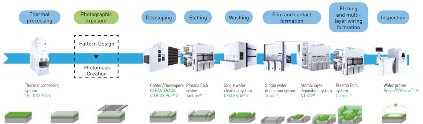
[Fig. 3 Semiconductor manufacturing (Front-end Process) and equipment]
