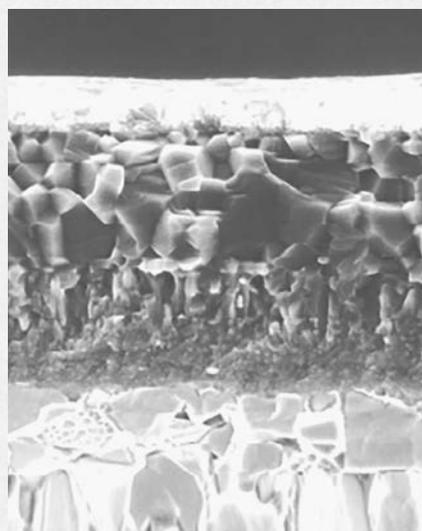
The Company worked on multi-layer coating using adhesion technology in the mid-1970s. Ti compounds with high wear resistance and a multi-layer structure of chemically stable  $Al_2O_3$  satisfied the conditions required for machining in a well-balanced manner. Research on high-intensity adhesion of these two layers confirmed that using TiCO layer as the middle layer maximized the adhesion. Using this technology, the Company released U77 in 1977.
