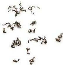
With controlled vibration frequency = 1.25/rev
