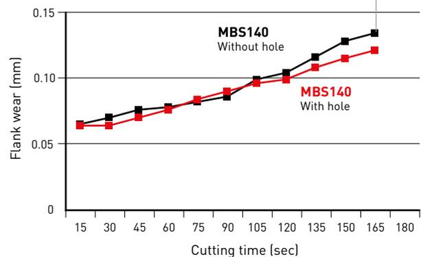
Vibration occurred when using an insert without hole after 165 sec due to high cutting loads.
