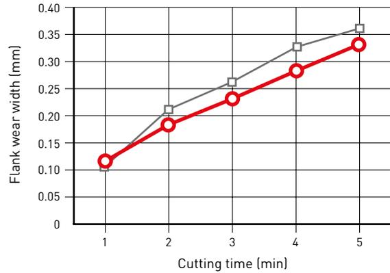
Stable flank wear is maintained compared to conventional products. Ideal for continuous cutting.
