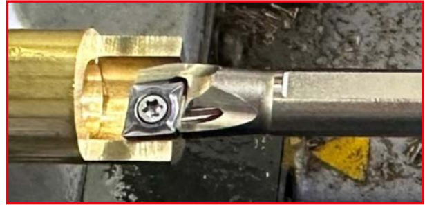
Dimple Bar Minimum machining diameter of 10 mm
